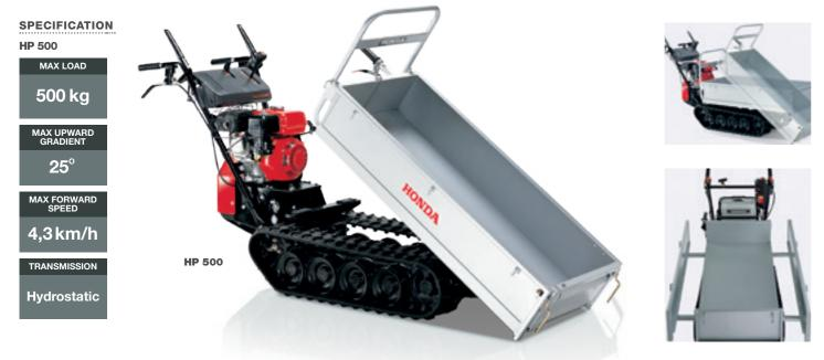
Our power carriers are flexible - simply adjust the bed for different sized materials
